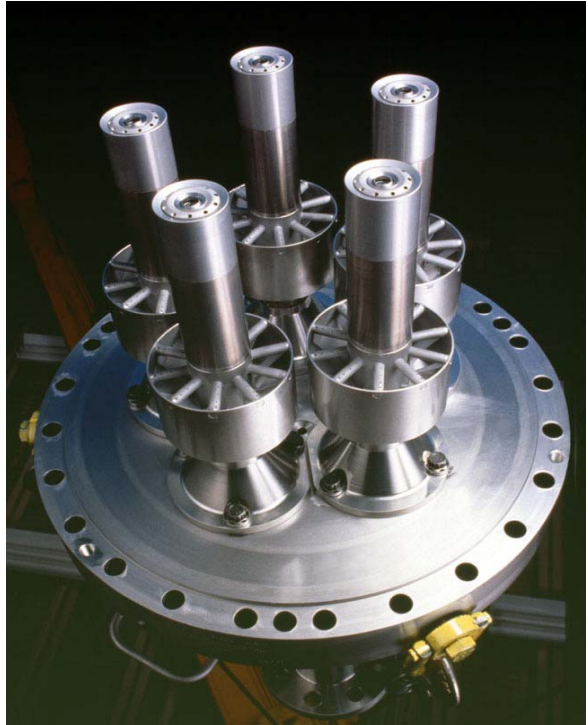
Fig. 31. DLN (dry low NOx) combustor (Source: GE Power Systems)
