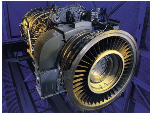
Fig. 33. A GE LM6000 partially assembled. (Source: GE Power Systems)
