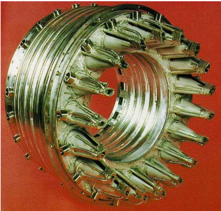
Fig. 32. The SGT-600 dry, low-emission (DLE) combustion system Source: Siemens Westinghouse
