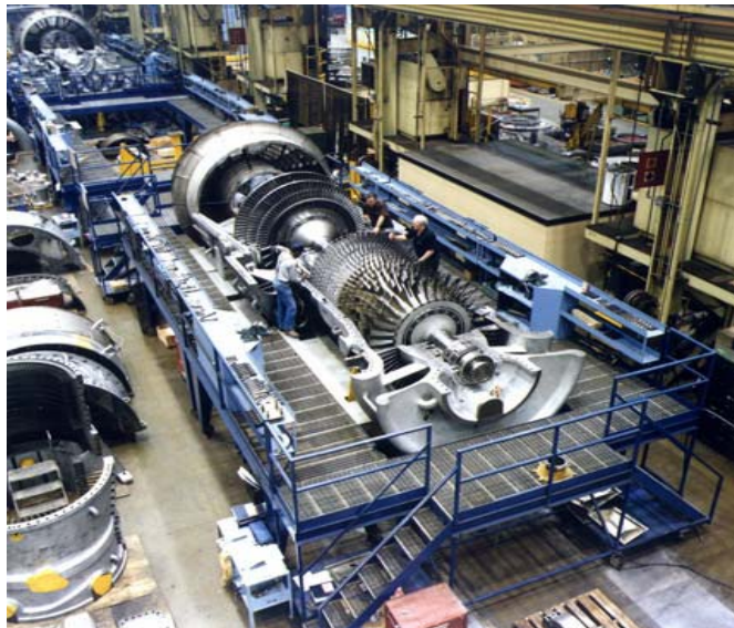
Fig.18. GE Frame 7F during manufacture/test showing rotor in half the casing (Source: GE Power Systems)
