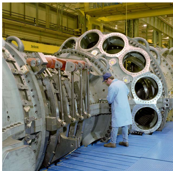
Fig. 30. GE 9H partial combustion module during manufacture (Source: GE Power Systems)
